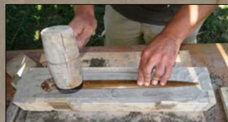
Step 3. Pushing the sword model into the sand to obtain the shape
