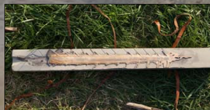
Fig. 5-6: deterioration of experimental stone moulds due to frequent utilization.
