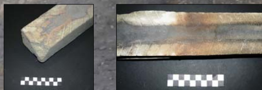
Fig. 5-6: deterioration of experimental stone moulds due to frequent utilization.
