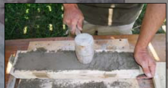
Step 1. Filling one of the two wooden boxes with calcareous fine sand and pressing it with a hammer
