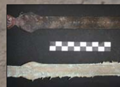
Fig. 9: notice the degree of precision in the edges of the two blades made out from sand casting (on the top) and from sandstone casting (below).
