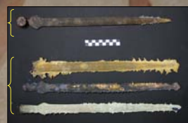
Fig. 8: one sword from sand casting in comparison with three swords from stone moulds.
